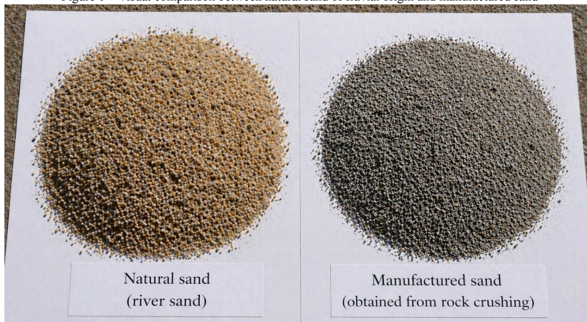
Figure 1 – Visual comparison between natural sand of fluvial origin and manufactured sand
