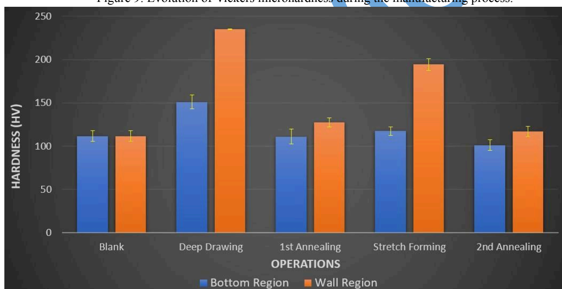
Figure 9: Evolution of Vickers microhardness during the manufacturing process.
