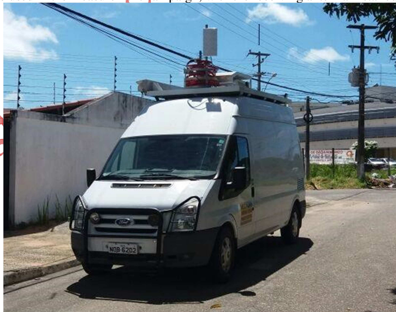
Figure 1 –Vehicle used in the measurement campaign, with the receiving antenna installed on its roof
