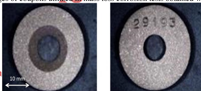
Figure 1 – Typical images of coupons utilized in mass loss corrosion tests obtained with 8 times magnification
